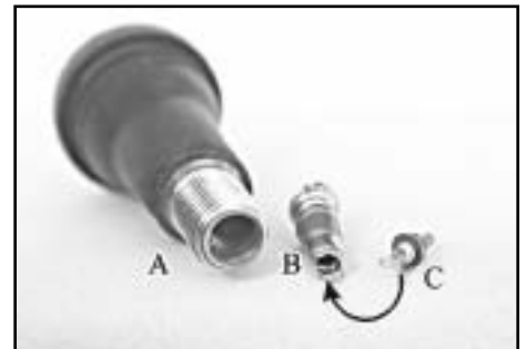
Figure 4 Air passage holes in a tire valve stem without the valve core (A) and within the valve core (B).
