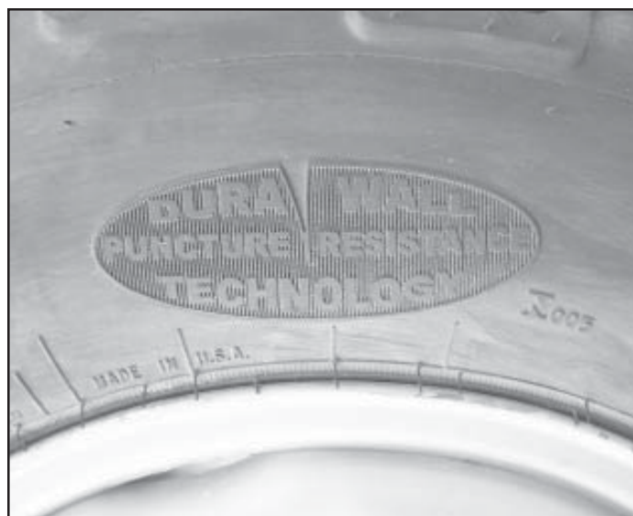
Figure 2 Silica compounds in the sidewall make the MT/R Durawall very tough!
