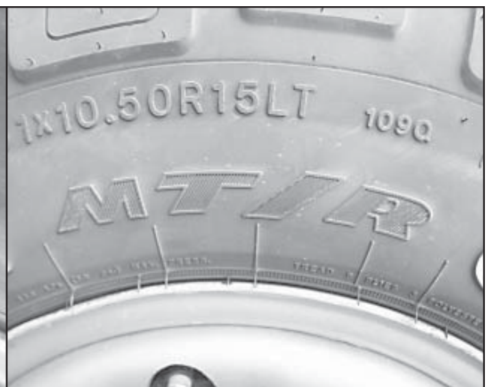
Figure 3 When you see the MT/R on the tire, you are assured of 3-ply sidewalls.
