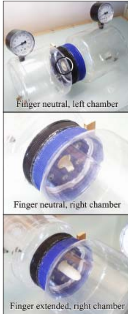
Figure 2 The top two photos show the finger in the neutral position. The bottom photo shows the finger extended (lower pressure in this chamber).
