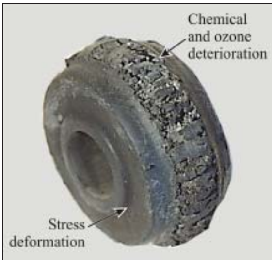
Figure 1 Factory rubber bushings deteriorate with exposure to the elements and stress.
