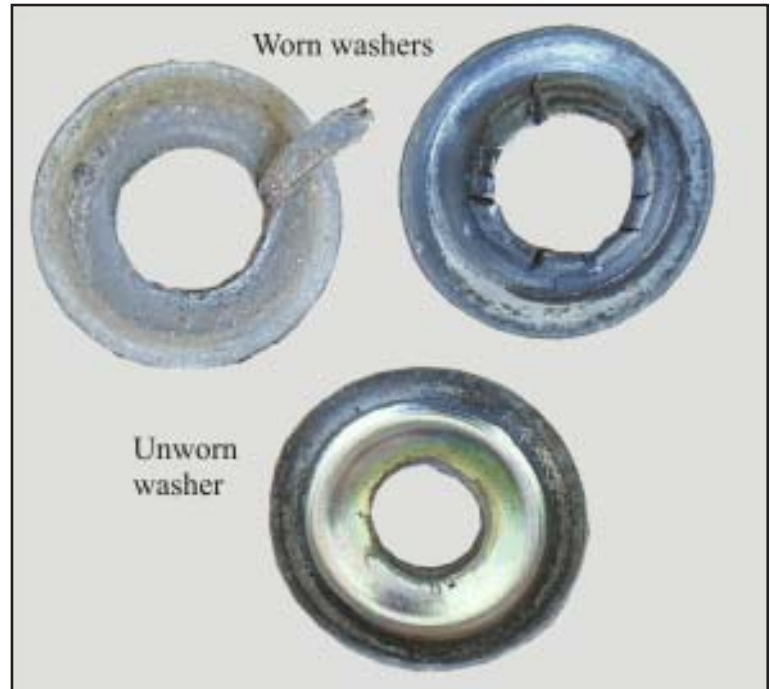
Figure 2 Rubber bushing deterioration leads to washer failure.
