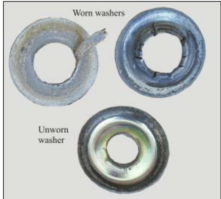
Figure 2 Rubber bushing deterioration leads to washer failure.
