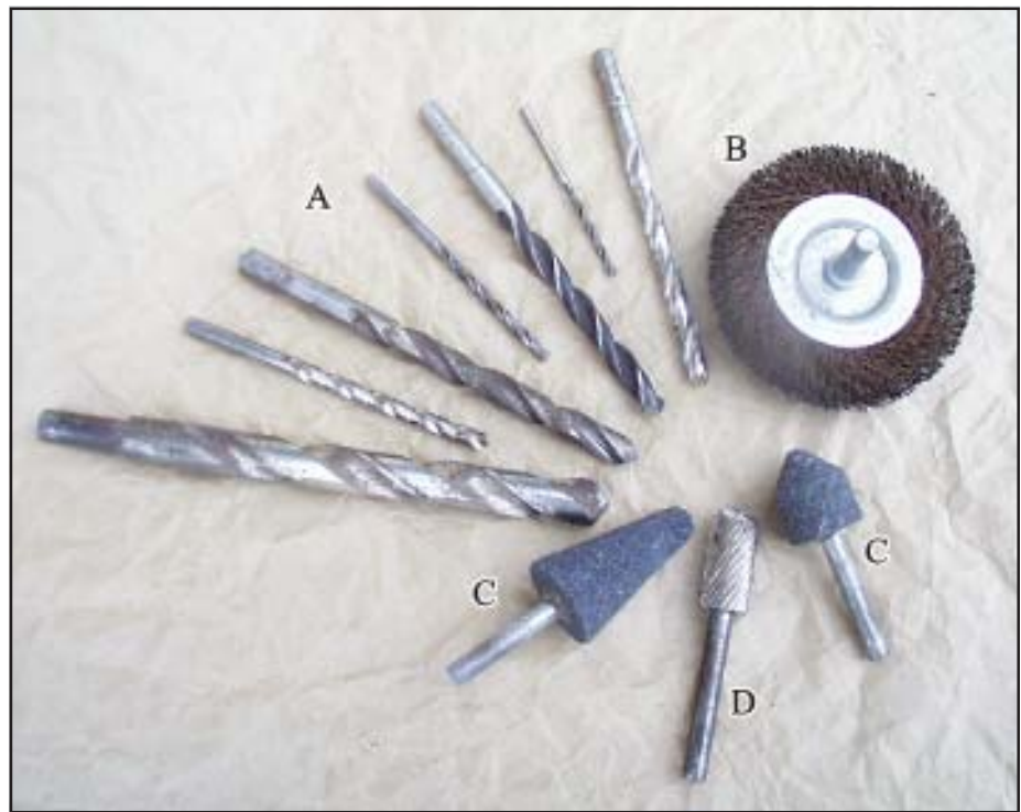
Figure 5 Getchaback drills: A) 1/2 to 1/16 inch drill bits; B) Wire brush; C) Grinding stones; D) Rotary file
