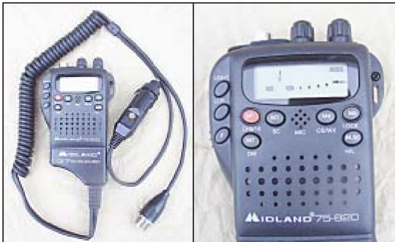
Figure 1 Mobile converter (left) and keyboard/display panel (right)
