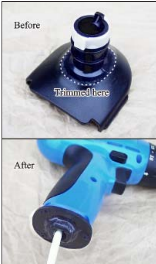
Figure 3 Project drill power connector conversion
