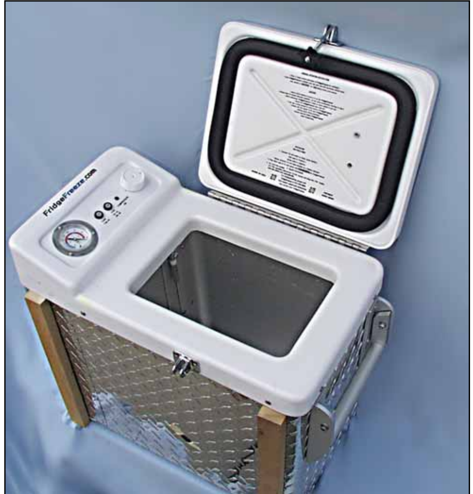
Figure 1 20 liter FridgeFreeze with circulation, spacer boards added by Bill Wilkinson.
