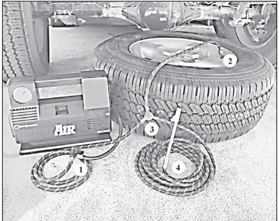
Figure 1 A COYOTE AIR ROBBER with TruckAir compressor and spare tire "tank" connected. The tire would normally be up, out of sight. Photo by Harry Lewellyn
