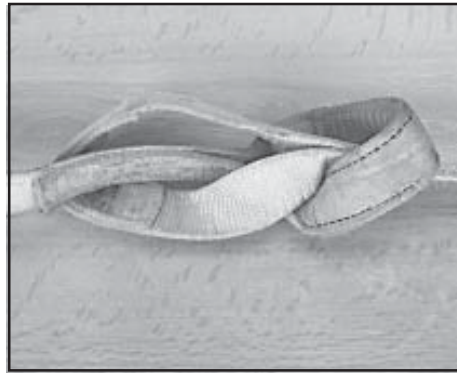
Figure 13. Loop-through-loops can become permanent! Photo by Lewellyn
