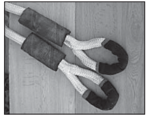
Figure 5 Lower radiator hose "damage protectors" on towline. Photo by Lewellyn
