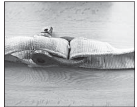
Figure 14. WRONG! Never use a shackle (cannonball) to attach two yankers!
