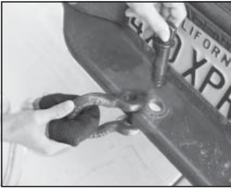
Figure 7. Loop shackle through Towline eye and attach to trailer hitch ball hole.
