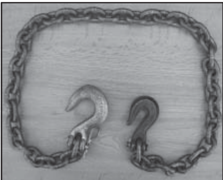
Figure 8. Three-foot Coyote chain with choke hook on left and grab hook on right
