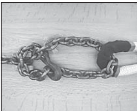
Figure 10. WRONG! A grab hook attached this way stresses the line.
