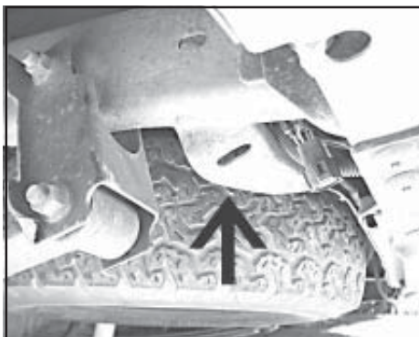
Figure 3 Rear horizontal D-hole near spare tire. Photo by Lewellyn
