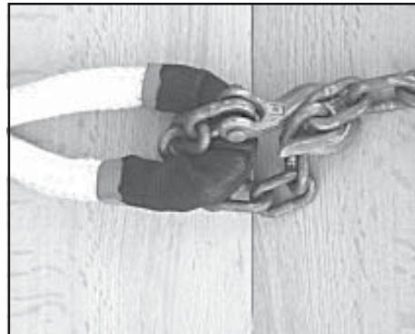
Figure 9. CORRECT! A grab hook attached this way is best.
