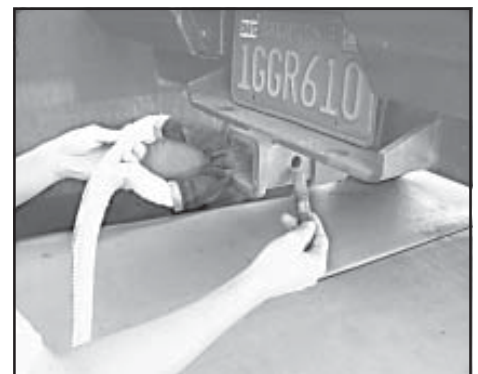
Figure 6 Insert Towline eye into class III trailer hitch and pin. Photo by Lewellyn
