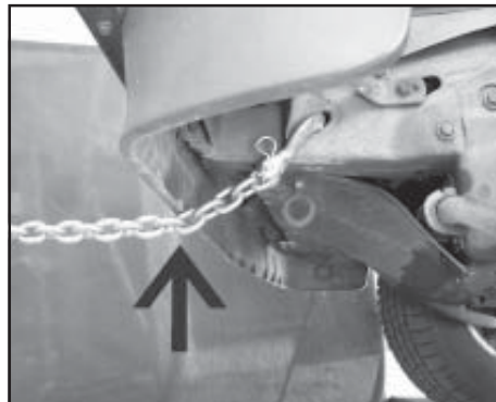
Figure 4 Choke hook in vertical D-hole, but note potential air dam damage.
