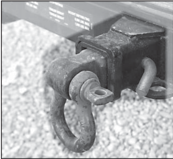
Figure 6 A class III towing insert Photo by Harry Lewellyn
