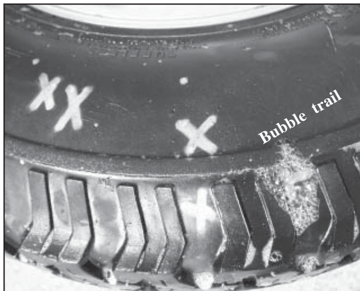
Figure 1 Xs marks four holes and the bubble trail (right, middle) confirms another.
