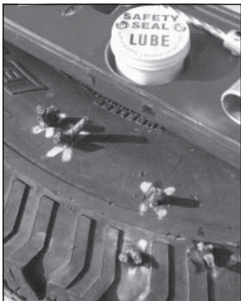
Figure 2 Five plugs ready to trim
