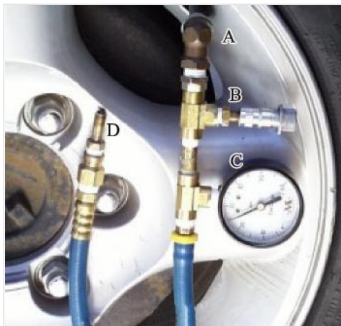
Staun Tyre Deflator test fixture.
