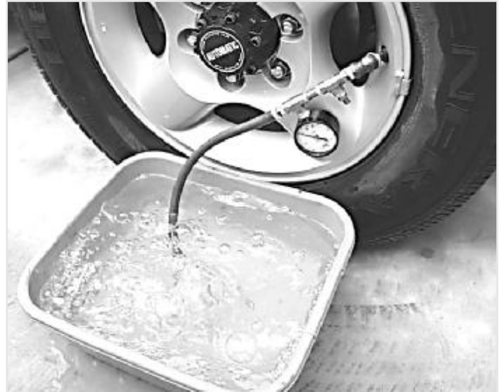
Water test: Valve deflating.
