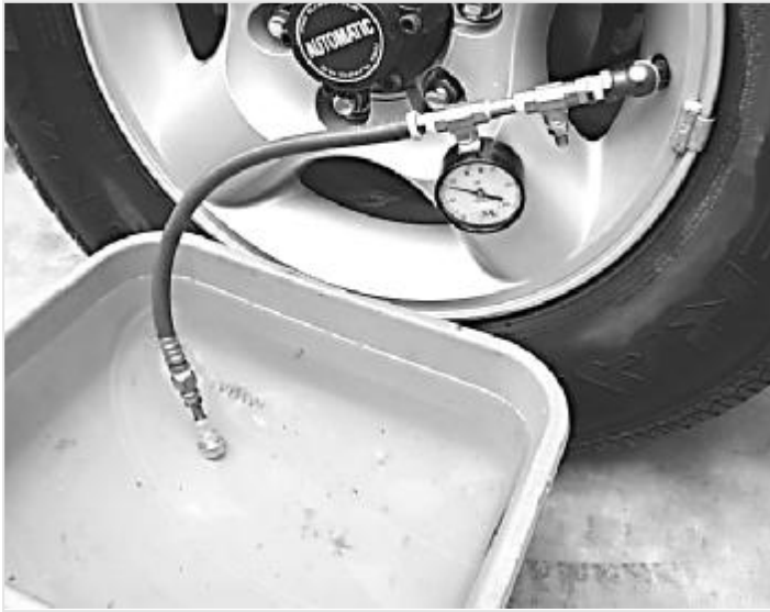
Water test: No evidence of leakage.
